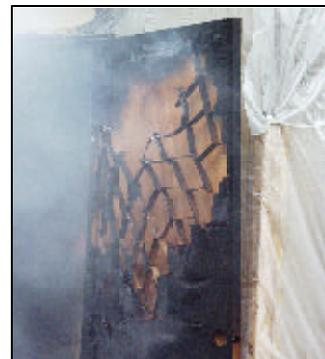
Standard inside door after 15 minutes of fire. Notice the room side of the door is still intact.
